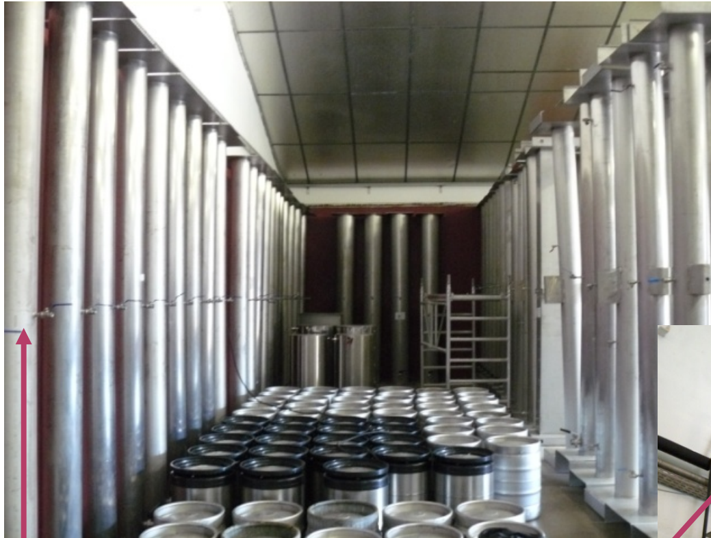
Cigar-shaped stainless steel tanks with mid-tank sampling
